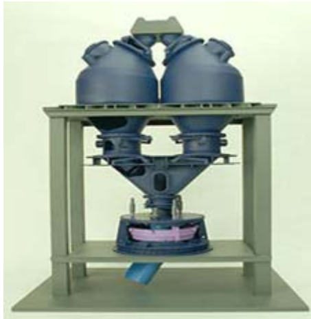
Figure 2: Bell Less Top charging system
