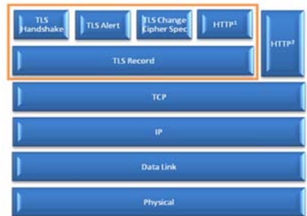
Figure 4: SSL/TLS Protocol Layers
