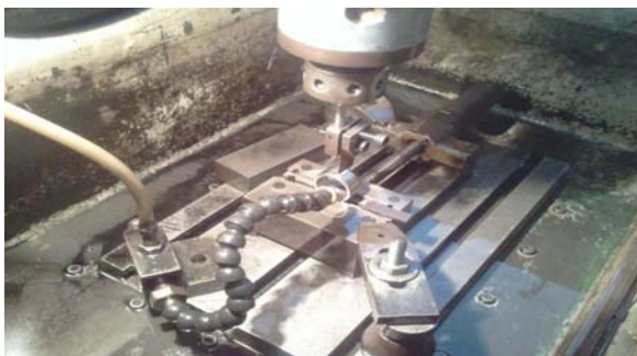
Figure 5.3: Introducing defect on the inner race
