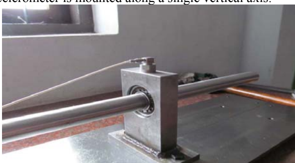
Figure 5.5: Accelerometer mounted on the housing
