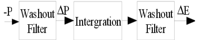
Figure 4.3: Obtaining the input signals for fuzzy controller
