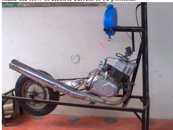
Figure 8: Experimental Setup – Two Wheeler Silencer with TEG
