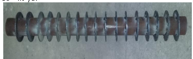
Figure 1: Mild Steel pipe with Fins
