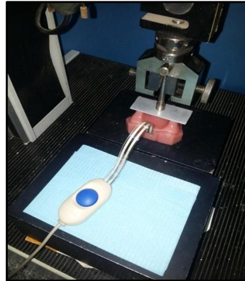
**Figure 4:** A perpendicular static load applied to the overdenture using universal testing machine.
