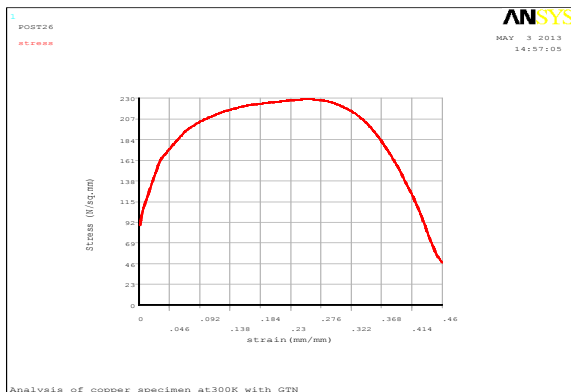
Figure 4: Engg. stress strain plot of copper specimen with GTN model at 300 K
