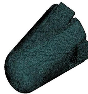
Meshed capsule within the flow domain
