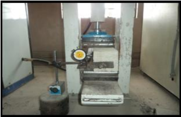
Figure 1: Yoke set up for load-deflection measurement.
