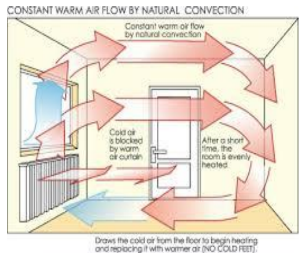
Figure 9: Heat transfer in a free convection
