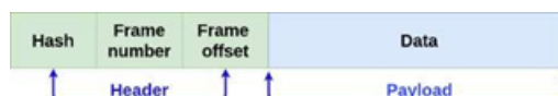
Figure 4: Represents the frame data structure. The header contains the digest of the entire frame, frame number, and flash offset location. The payload contains corresponding data for each frame.
