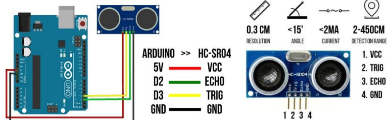
Figure 5: Ultrasonic sensor with pin details
