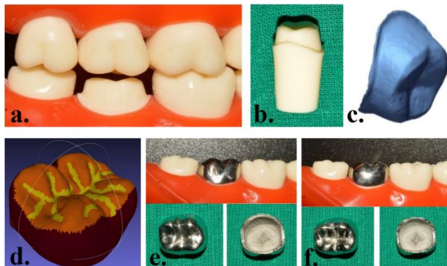
Figure 1a: Tooth preparation done on a lower right molar on a typhodont, 1b: Prepared die, 1c: Die scan, 1d: Design of the 3D CAD Model on the CAMbridge software, 1e: Co-Cr crown manufactured by Direct Metal Laser Sintering method, 1f: Co-Cr crown manufactured by Milling method)
