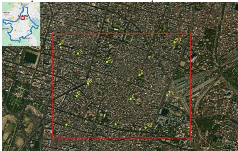
Figure 1: Location Map of Study Area. The green dots are used to measure SVF using fish eye lens and SVF mapping tools and validate to check accuracy with the observed SVF values of UMEP QGIS and proposed python script
