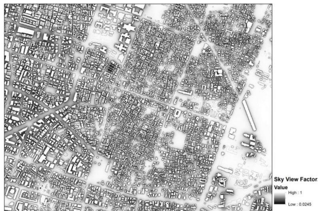
Figure 6: Sky View Factor Map prepared in QGIS using UMEP plugins. Spatial resolution is 10 meters
