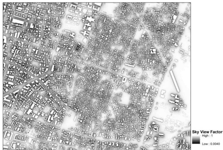
Figure 3: Sky View Factor map prepared using Python script. Spatial resolution is 10 meters
