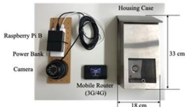
Figure 6: IoT gadget setup for moving object detection and data collection.
