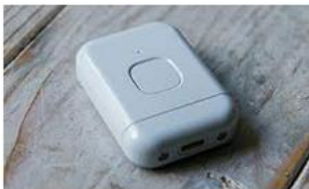
Figure 8: ELTRES, the LPWA wireless adapter.
