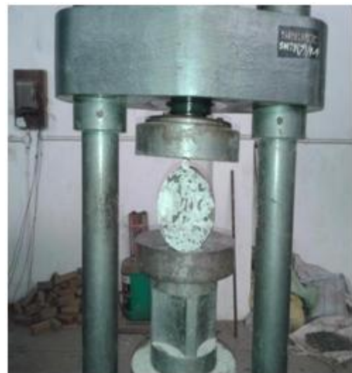
Figure 6: Showing failure of the cylinder
