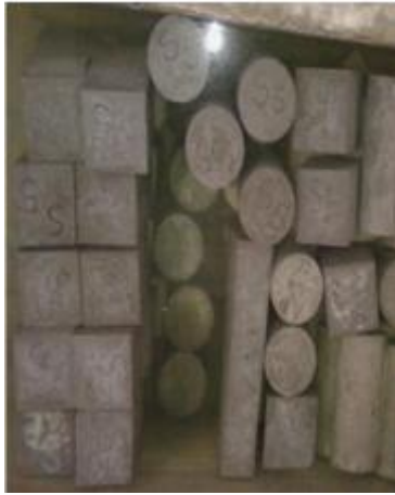
Figure 5: Showing curing of the cube
