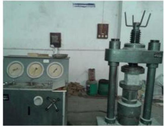
Figure 2: Showing compression testing machine
