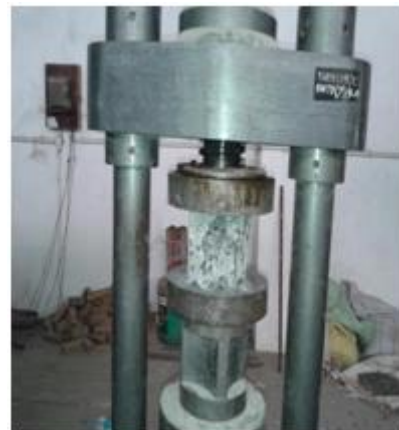
Figure 3: Showing failure of the cube
