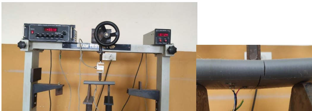
Figure 3 (a): The experimental set-up used for the testing of honeycomb-structured 3D printed sandwich panel
