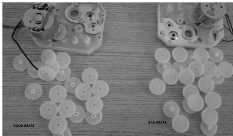
Figure 11: Impeccable and Defective gears used to extract sounds for testing
