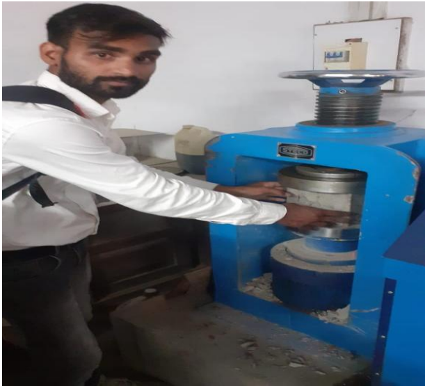
Figure 6: Compressive Test of Blocks through Digital Testing of Compressive Machine
