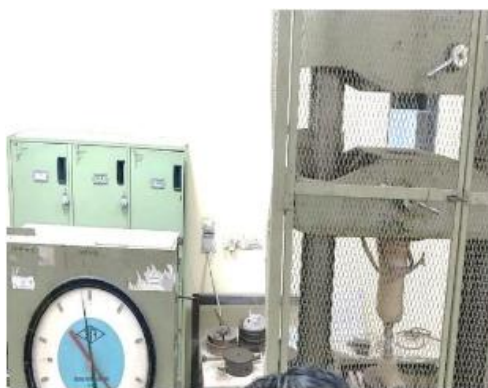
Sample A: Glass fiber polyester composite socket handles the compression of 18.35 kN.
