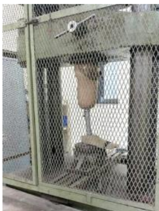
Sample A: Glass fiber polyester composite socket handles the compression of 18.35 kN.
