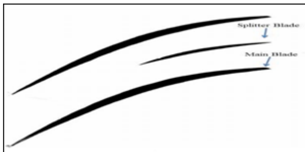
Figure 4: Wennerstrom's tip section blade and passage geometry
