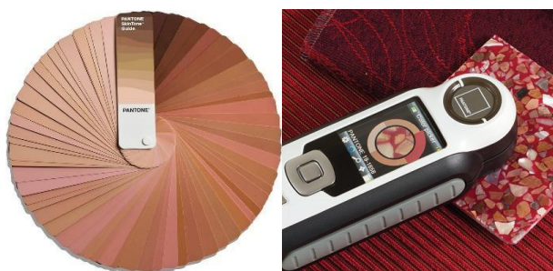
Figure 1 on left Pantone color guide, one of the most famous tools in color matching, on the right digital device for color identification
