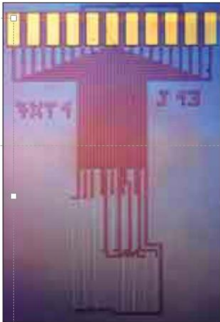
Figure 5: A magnetic Field Sensor made of GMR multilayers (iron nickel with Silver) for an angular encoder
