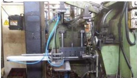
Fig 1.3 Design of Pneumatic Pick and Place Automation for Groove Grinding Machine [10]
