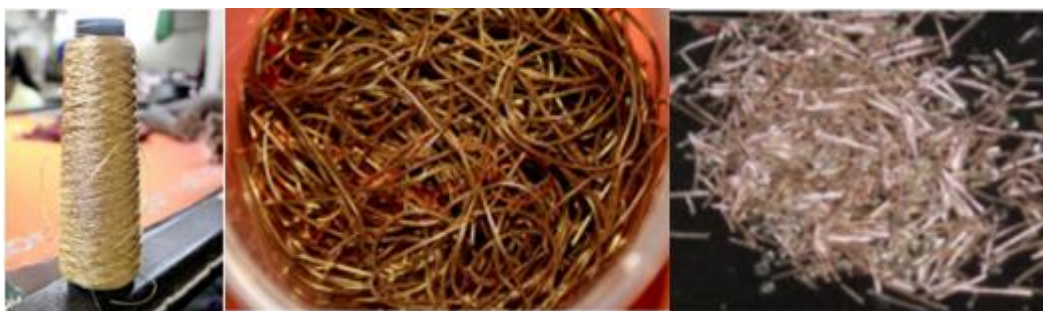
Figure 1 (left) Metallic threads that are originally made out of cotton and coated with metallic dyes. (center) Metallic wires are made out of alloy and coated. (right) dabka and sitara are made out of plastic or cheaper substitutes with a metallic coating
