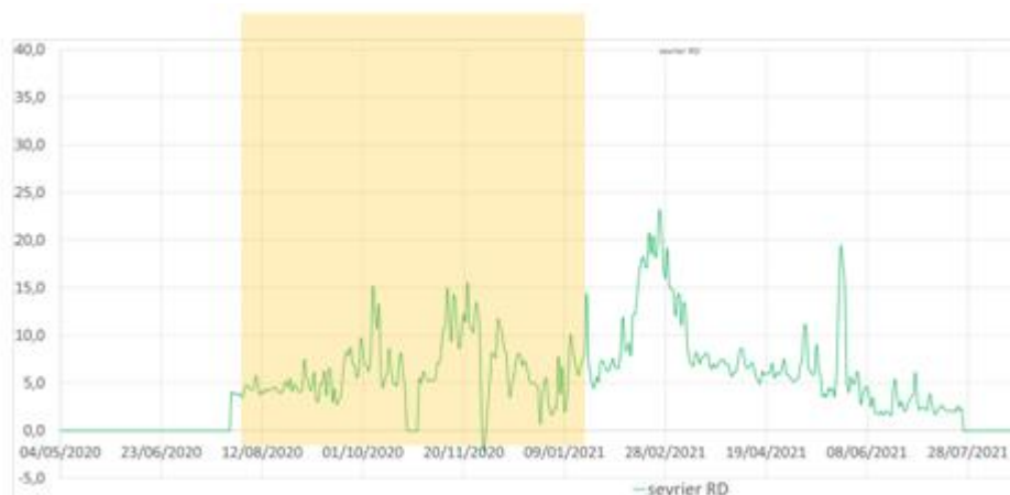
Figure 20b: PM level measured by a second air monitoring micro - station situated on a departmental road below the campsite (based on daily averages).
