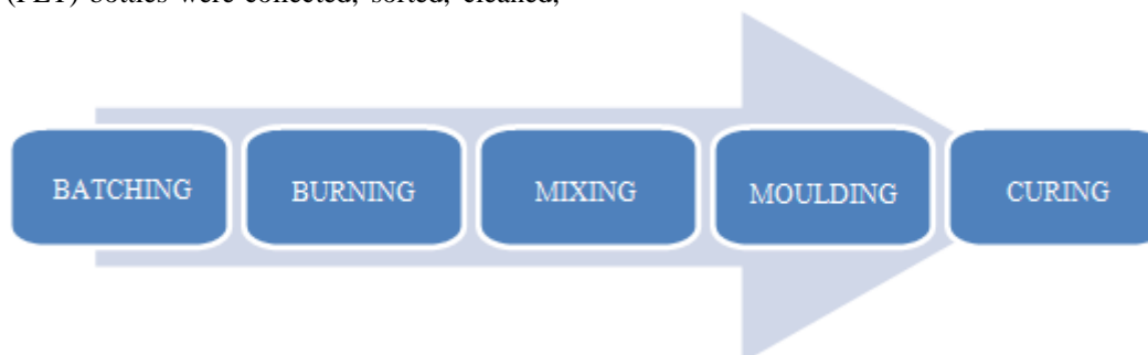
Figure 1: Procedure of Casting Plastic Sand Bricks
