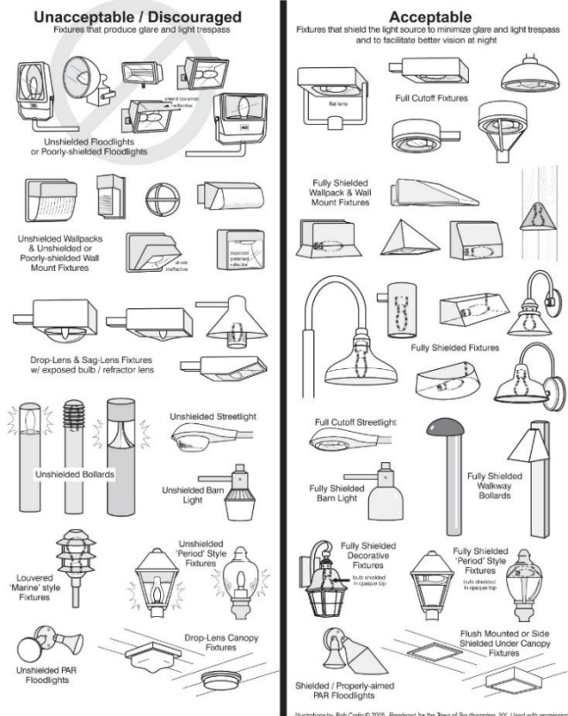
Differences between unacceptable and acceptable lighting fixtures
