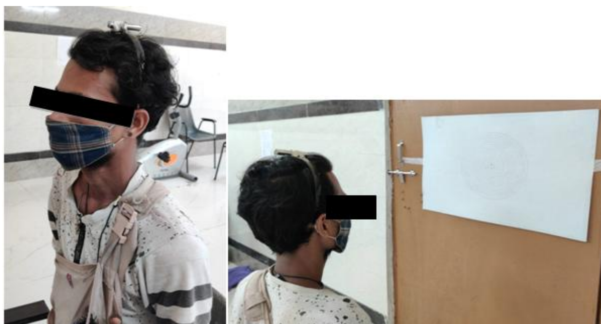
Fig 1 and 2: Subject wearing headband with a laser beam device attached, seated blindfolded on a chair with backrest and Target with concentric circles at 90cm distance.
