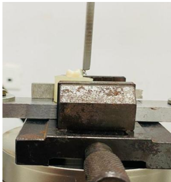
Figure 3: Testing of Shear Bond Strength of a specimen of group A (white)
