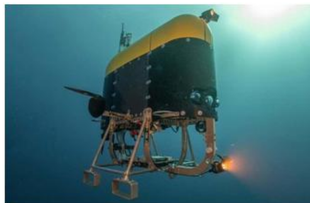
Figure 4: Aquatic predators tracking robot - Mesobot
