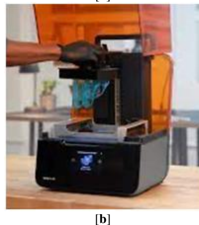
Figure 4: [a] SLA sketch, [b] SLA machine [27]
