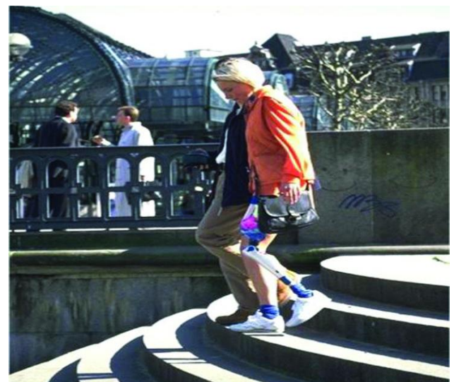
Figure 8: The Otto Bock C - Leg with computer - controlled knee and integrated motion and force sensors to optimise hydraulic damping, making both walking and stair descent easier. (Picture courtesy of Otto Bock)
