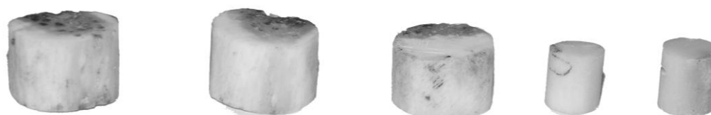
Figure 2: Sample for the determination of compressive strength
