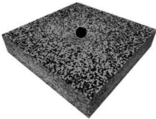
Figure 36: Skin model and the indenter that represent the durometer, after moving indenter down by 1mm
