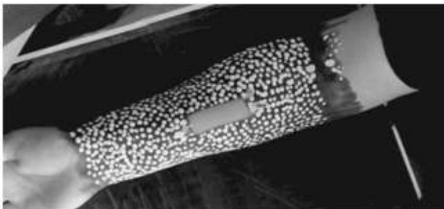
Figure 14: The dotted pattern applied over the whole volar surface of the forearm. Only the region of sticker is void from the pattern.
