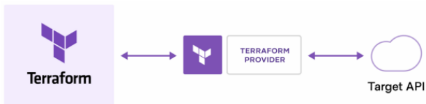
Figure 2: Terraform actions go through a provider module to translate into API calls specific to that provider
