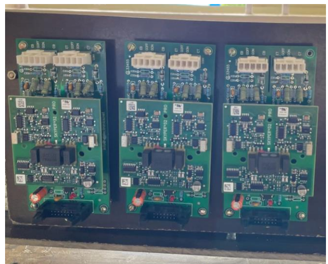
Figure 5: Driver Circuits fixed on board
