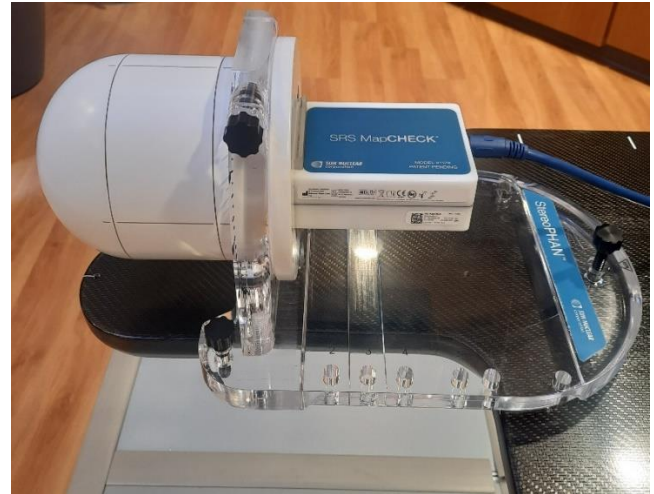
Figure 6: Patient Specific QA with SRS MapCHECK and StereoPHAN Phantom.
