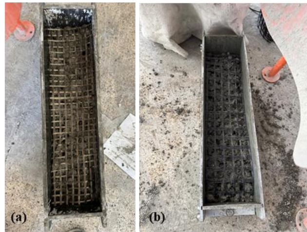
Figure 1: Placement of geogrids in the molds: (a) Basalt geogrid, (b) PET geogrid
