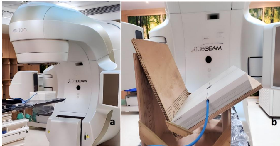
Figure 1: Phantom setup for a) normal beam incidence; b) oblique beam incidence to measure surface dose
