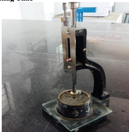
Figure 7: Final setting time
