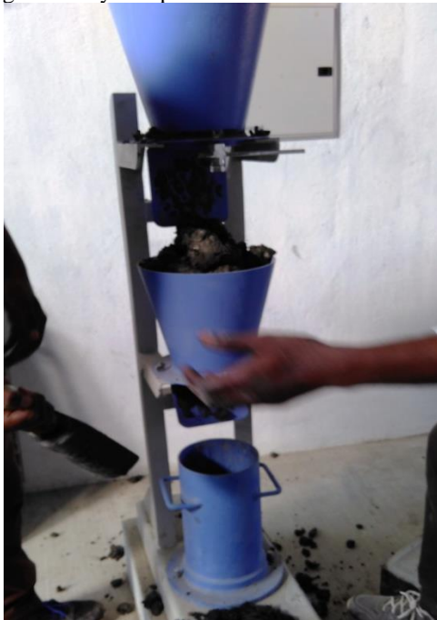
Figure 14: Compaction factor test
