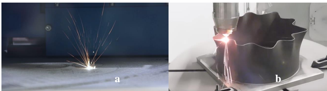
Figure 1 (a) An SLM machine while printing, and (b) A BeAM DED 3D printer depositing and melting metal powder with a dual-purpose print head [11]
