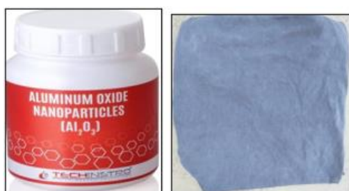
Figure 7: Aluminium Oxide Nano Powder (25gm) and Black Cotton Wick used in the experiment
