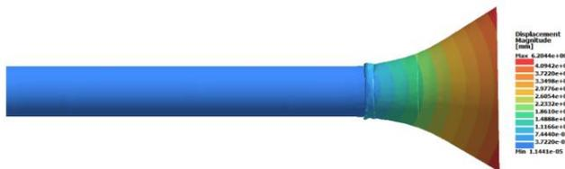
**Figure 15** This is the elastoplastic changes after final +X direction 75 newtons applied force.
