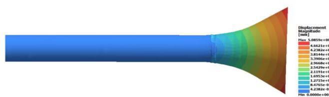
Figure 11: Displacement after unloading. You could recognize the deformation of the epiphyseal plate easily. Our knowledge about this change is nil in the human being.
