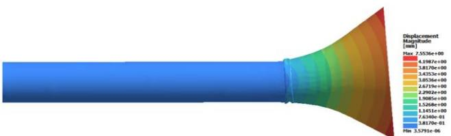
Figure 12: We had reversed the force and do a new deformation in an opposite direction to the initial deformation, and this is the resultant elastoplastic deformation.
