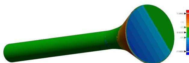
**Figure 19:** Comparison of the final deformation remained after unloading with the original input CAD
