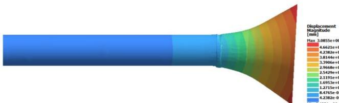
Figure 10: Elastic changes of the returning to initial status condition on the -X direction.
