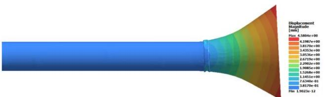
Figure 14: The remaining displacement after unloading. To complete the full cycle we had to return the model to its original position with 75 newtons in the +X direction.
