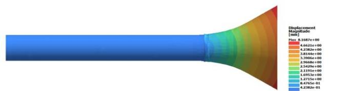
Figure 9: The previous model that resulted from the final unloading changes had been simulated with force on the -X direction. This is elasto-plastic changes.
