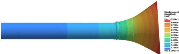
**Figure 16** This is the elastic changes after final +X direction 75 newtons applied force.
