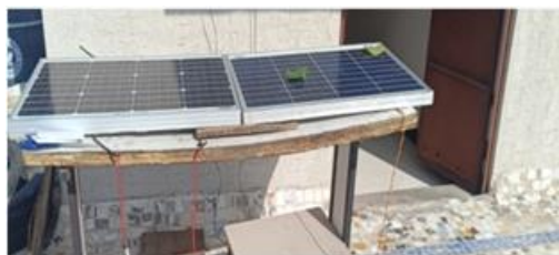
Figure 3: Tree leaves shading
