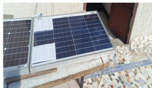
Figure 2: Concealing of two series associated cells
