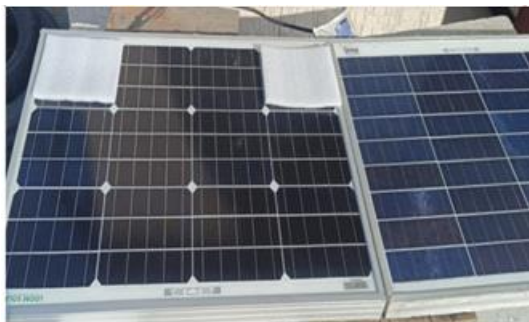
Figure 4: Card board shading for two parallel cells
