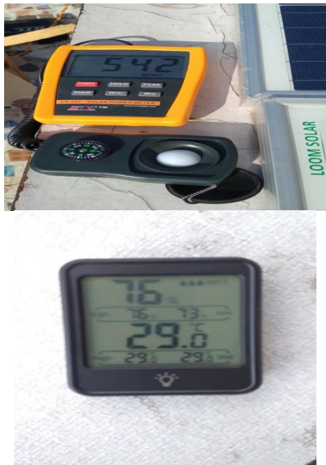
Figure 4: Instruments for measuring Insolation, Temperature and Humidity
