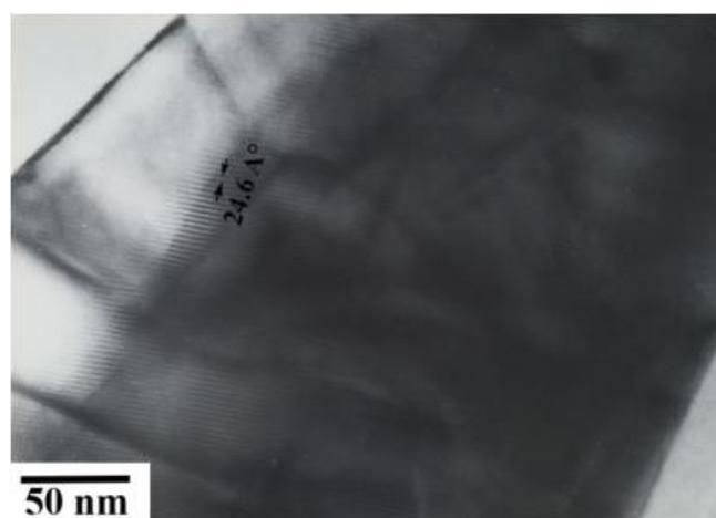
Figure 3 (a): Lattice planes of 2201 phase observed in sample No.2
