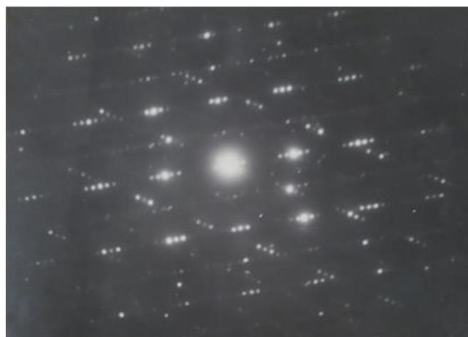
**Figure 4 (c):** SAD Pattern observed in Sample No. 3
