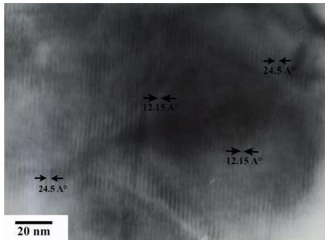
**Figure 4 (b):** Lattice fringes observed in Sample No. 3
