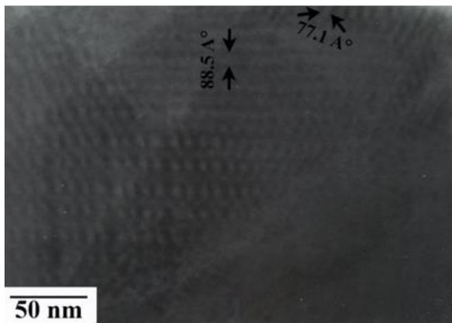
Figure 5 (a): Moire fringes observed in Sample No. 4
