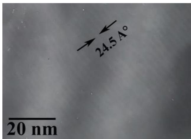
Figure 2: Lattice planes of 2201 phase observed in sample No.1
