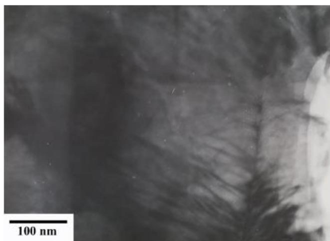
**Figure 4 (a):** Dislocations and Twinning observed in Sample No. 3
