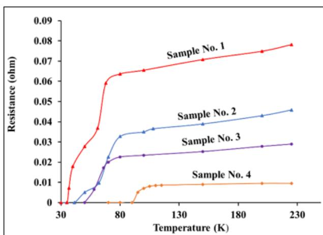
Figure 1: The resistance vs temperature characteristics of sample Nos. 1, 2, 3 & 4
