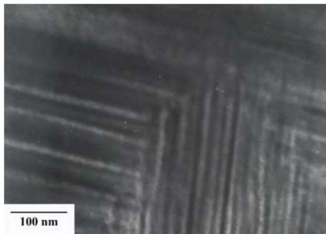
**Figure 3 (b):** Band Structure and Twinning observed in sample No.2
