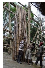
Figure: Vertical stacking after 7 days of soaking in boric acid or borax solution
