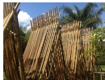
Figure: Being left to dry in the sun solution
