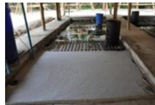
Figure: Bamboo culms being treated with borax powder
