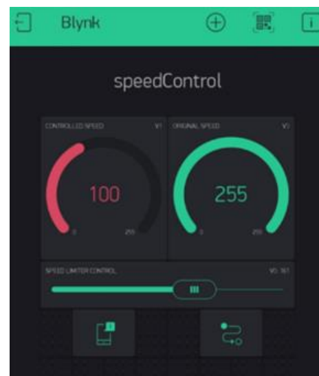
Figure 13: Working of Speed Control with slider control of blynk App
